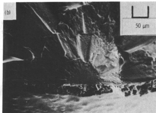
Figure 9 SEM of room temperature fracture of CNTD-SiC oxidized for 100 h at 1200° C, \sigma_f 146 ksi (1000 MPa).
